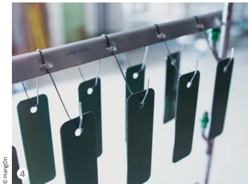
Figure 4: The HQL bar allows inserting a double hook so that the workpieces can be hung symmetrically.
